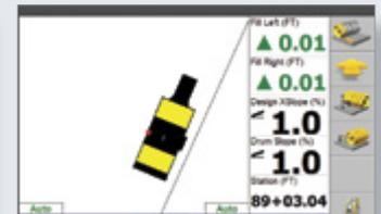
Guidance to grade shown to the operator in plan, profile, and cross section view
