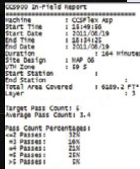
A printed in-field report showing pass count coverage
